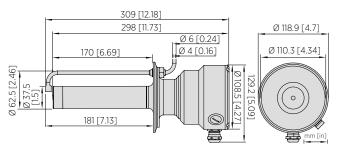
Dimensions PR53AP Sanitary 4", depth 170 mm, with wash nozzle
