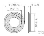
PR53AP tank bottom welding flange dimensions
