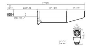
Dimensions of HMP80L (top) and HMP80N (bottom), side and bottom view
