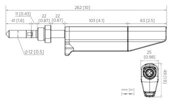
Dimensions of DMP80 series probes with G1/2" thread, side and bottom view
