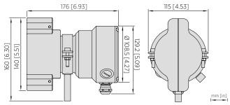
Dimensions PR53M tube fitting
