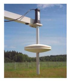
PTB210 paired with SPH10 static pressure head
