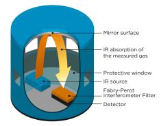
Structure of the CARBOCAP sensor
