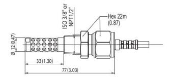
MMT317 probe, dimensions in mm (inches)
