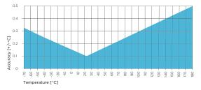
HMP8 temperature measurement accuracy over full range
