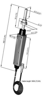
Probe dimensions in millimeters (inches)
