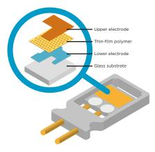
Structure of the HUMICAP sensor
