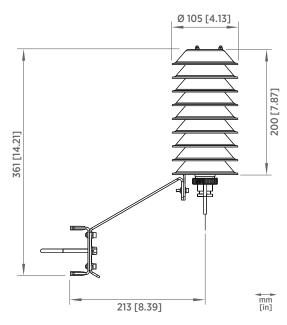
Solar Radiation Shield DTR502B dimensions
