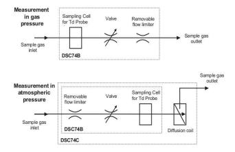
The DSC74B sampling cell enables the measurement of the sampled gas either in gas pressure up to 10 bar or in atmospheric pressure depending on the gas inlet and outlet. DSC74C is like DSC74B but with an additional coil to avoid back diffusion, the effect of surrounding moisture, in dew point measurements in atmospheric pressure.
