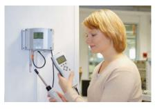
Handheld Humidity and Temperature Meter HM70 is ideal for field checking HMT330 transmitters
