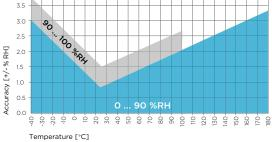
HMP8 humidity measurement accuracy as a function of temperature
