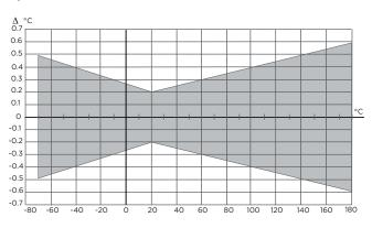
Temperature measurement accuracy over temperature range
