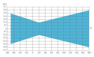
Temperature measurement accuracy over temperature range
