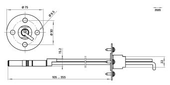
Duct installation kit 210697 dimensions with probe
