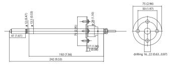
DMT345 Probe and Mounting Flange
