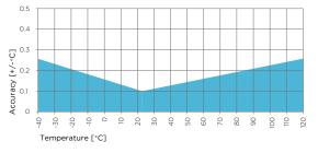
HMP9 temperature measurement accuracy over full range
