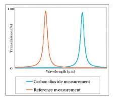
Example of carbon dioxide measurement. Both reference and CO2 absorption are measured in the same optical path
