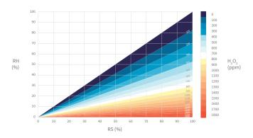
For example, at 20 °C and 500 ppm hydrogen peroxide, the humidity level 25 %RH is equivalent to 60 %RS. When this gas mixture starts to condense (relative saturation being 100 %), relative humidity is 45 %.
