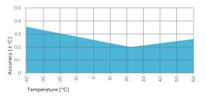
HMP1 temperature measurement accuracy over full range
