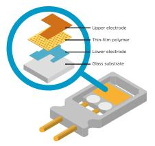
Structure of the HUMICAP sensor
