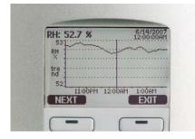
The display shows measurement trends and over four years of realtime measurement history. The display alarm allows any measured
