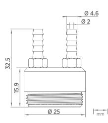
Flow-through adapter with gas ports ASM211697SP. Suitable for tubes with 4 mm inner diameter.
