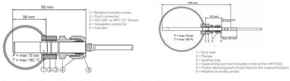
Pressure-tight Swagelok installation kits SWG12ISO38 with ISO3/8" or SWG12NPT12 with NPT1/2" thread (SWG6ISO18 with ISO1/8" or SWG6NPT18 with NPT1/8" thread for HMT337 temperature probe).
