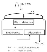
v<sub>t</sub> = terminal velocity of drop
