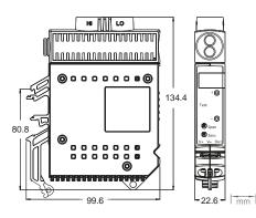
$\mathsf{PDT102}$  dimensions with process valve actuator and test jacks
