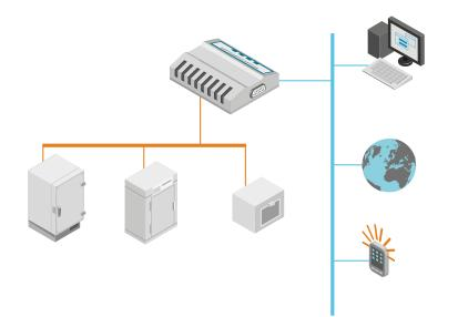
DL1016-1416 data loggers can be used with Vaisala software, either viewLinc or vLog, to download, display, and analyze environmental data.
