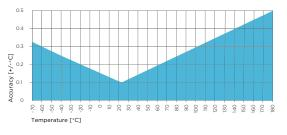
HMP7 temperature measurement accuracy over full range
