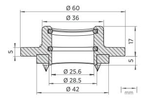
Probe mounting flange 243261SP dimensions, cross section
