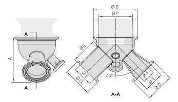
SEFC Sanitary Elbow Flow Cell, reduced inlet
