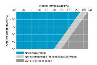
PR53AC process temperature, options Sanitary 2.5" and Type N (indicative)
