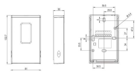
Dimensions (in mm) of GMW90 series transmitter cover (left) and mounting base (right)
