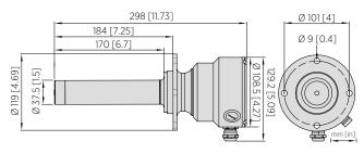
Dimensions PR53AP tank bottom flange, depth 170 mm
