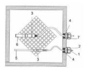
1 = PTFE sleeve 2 = Cable gland, example: AGRO 1100.12.91.065 3 = Stainless steel cable tie or similar fastener 4 = To be sealed (silicone) 5 = Temperature probe 6 = Relative humidity probe 7 = HMP247CG, Cable gland AGRO (available from Vaisala)
