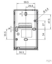
Dimensions of HMW90 series transmitter cover (left) and mounting base (right)
