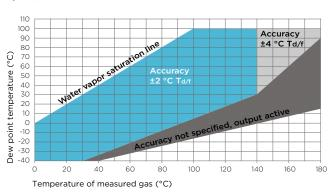
Dew point accuracy vs. measurement conditions
