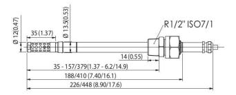
MMT318 probe, dimensions in mm (inches)
