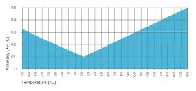
HMP5 temperature measurement accuracy over full range
