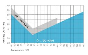
Humidity measurement accuracy as function of temperature
