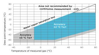
Dew point accuracy vs. measurement conditions
