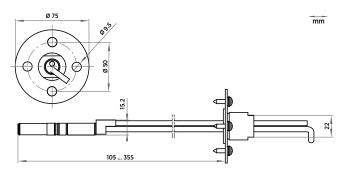
Duct installation kit 210697 dimensions with probe
