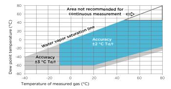
Dew point accuracy vs. measurement conditions
