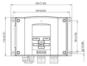
DMT345 and DMT346 Transmitter Housing
