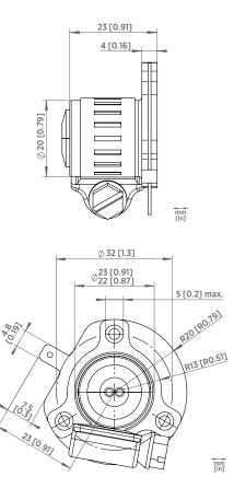
Probe mounting flange, side and front view
