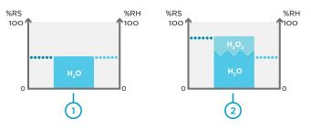
Space without H<sub>2</sub>O<sub>2</sub> vapor. When H<sub>2</sub>O<sub>2</sub> vapor is not present, relative saturation equals relative humidity.
