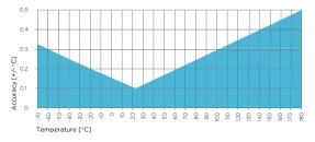
HMP4 temperature measurement accuracy over full range
