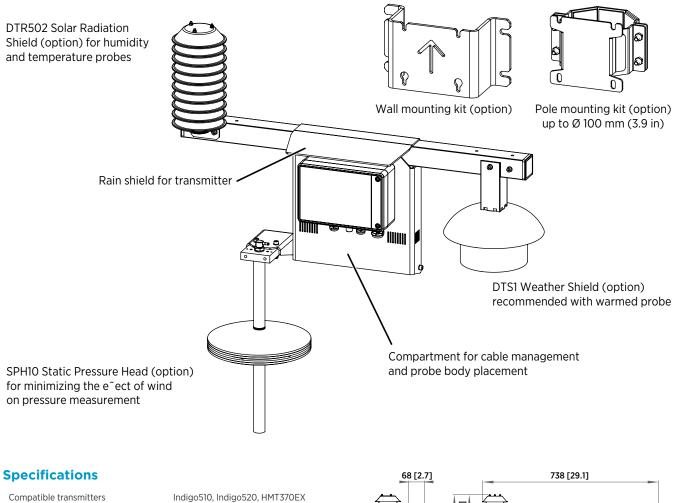
Compatible transmitters Compatible solar radiation shields Weather shield for heated probe Static pressure head Weight of mounting plate, probe compartment, and support bar Material of mounting plate, probe compartment, and support bar DTR502, DTR13, DTR250 DTS1 <sup>1)</sup> SPH10 <sup>1)</sup> 1.5 kg (3.3 lb)
