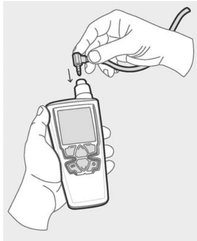
Snapping a connector to the HM40 indicator to read the measurement results.
