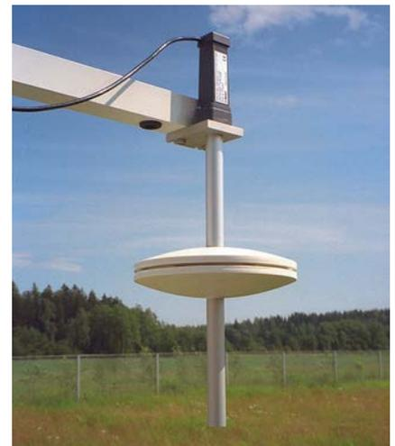
PTB210 paired with SPH10 static pressure head
