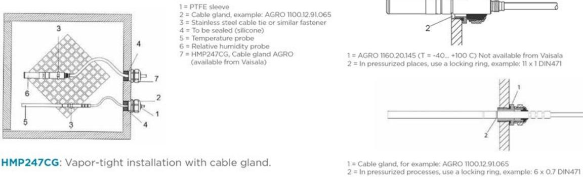
**HMP247CG:** Vapor-tight installation with cable gland.
