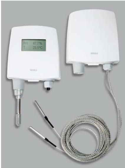
Vaisala Wi-Fi Data Logger HMT140 is designed for humidity, temperature, and analog signal monitoring in warehouses, freezer and cryogenic farms, laboratories, blood banks, and many other applications.
